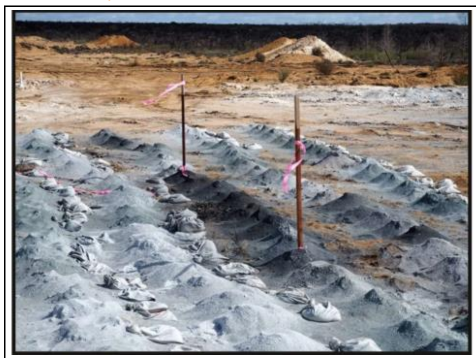
Figure 10: Massive sulphide intersections (128-138m marked by wooden pegs; NRRC124 R/C Drill piles)
